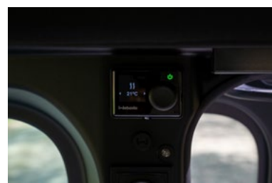
Chauffage gazoil 2000W
