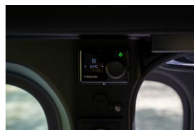
Chauffage gazoil 2000W
